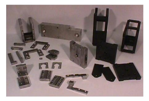
Sampling of Weldments, Machined Details, with Black Oxide and no Finish
