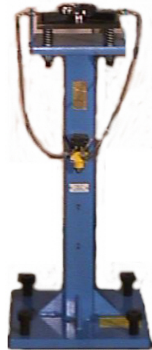
Robot Hand-off Between Cells Floor Support Frame Shown
